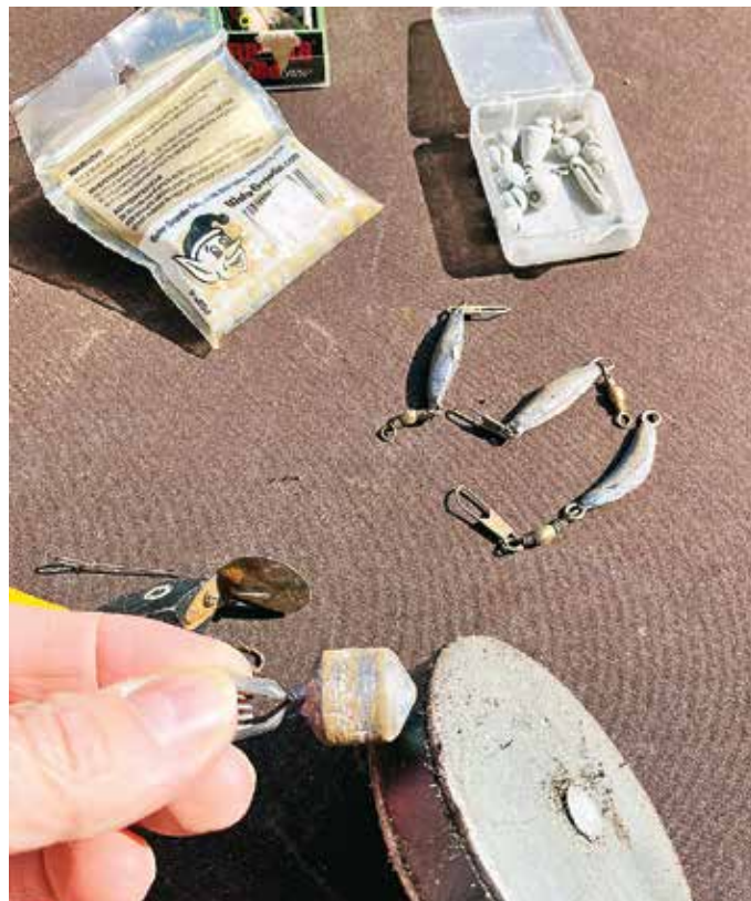
Using a magnet to test for lead
